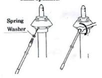
⑤Attach disk element and spring washer to disk base. After setting by hand then fasten firmly by 7mm spanner.
