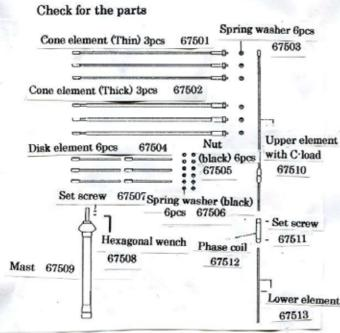
3All 6 pieces of cone element should be mounted. [note] Please attach thin cone element and thick element alternately. Two kinds of cone elements are included. One is thin cone element and another is thick cone element.
